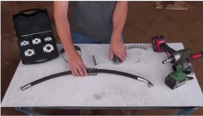
1. Place clamp over leak.
