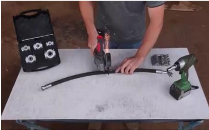
1. Cut hose center of the leak.
