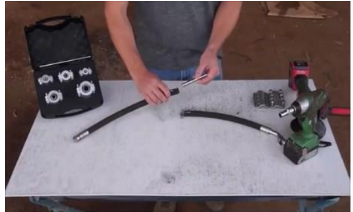
2. Insert joining barb.
