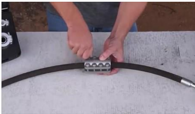
5. Finger tighten bolts.
