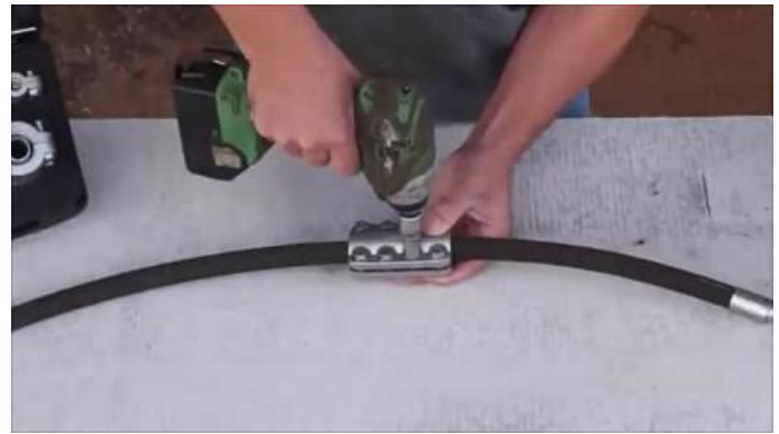
6. You will need a 12mm socket spanner to tighten bolts, tighten bolts evenly.
