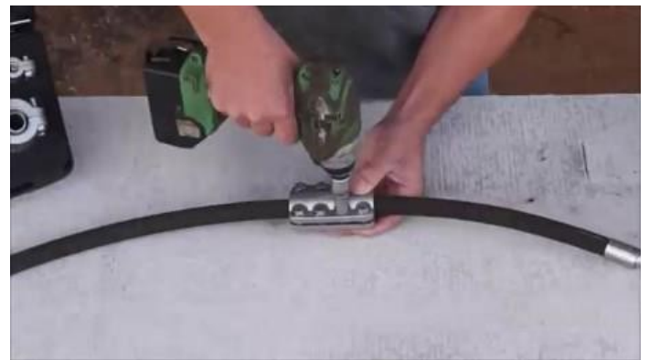
4. You will need a 12mm socket spanner to tighten the bolts.
