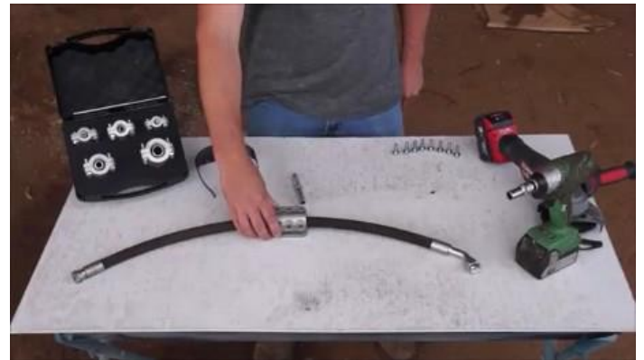
2. Ensure the leak is in the center of the clamp.
