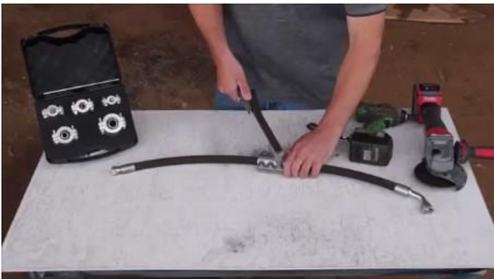
5. Tighten the bolts evenly as per the operator's manual (40Nm).
