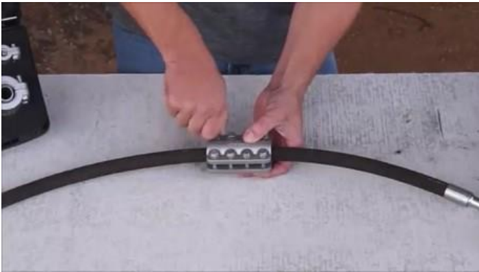
3. Finger tighten the bolts
