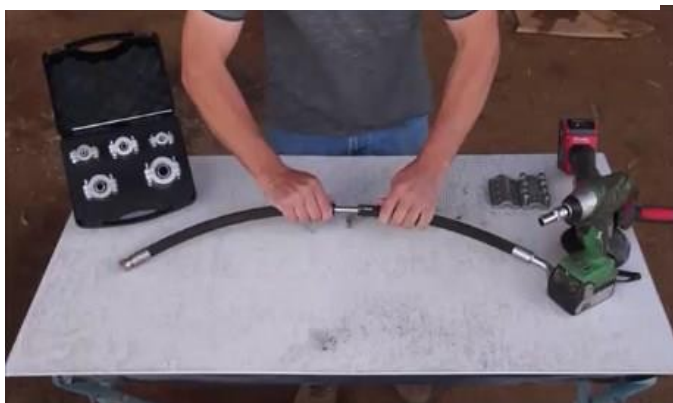
3. Join hoses to the center of the joining barb.
